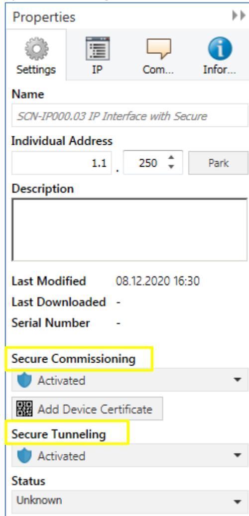
Figure 3: Secure Commissioning/Secure Tunneling
